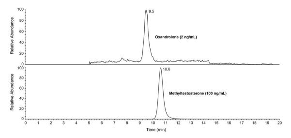
Figure 2. Chromatogram of oxandrolone (top) and methyltestosterone (bottom) peaks. The oxandrolone peak is at a concentration of 2 ng/mL (lower limit of quantitation) and methyltestosterone peak is at 100 ng/mL.
